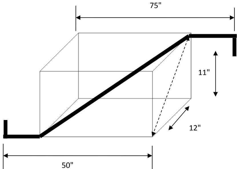
**Task 2:** Calculate the setback and diagonal for the following pipe schematic using a
